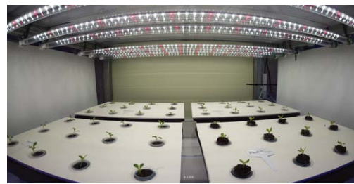
Normal Full Spectrum LED Full White (450nm) + Red (660nm)
