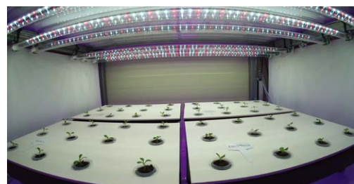
Plant-centric Spectrum LED (LM301H EVO Mint White) Mint White (437nm) + Red (660nm)
