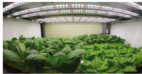
Normal Full Spectrum LED Full White (450nm) + Red (660nm)
