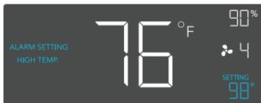
Note that alarm triggers can only activate in AUTO, ON, or TIMER Mode. Please leave ALARM SETTING to arm the controller.
