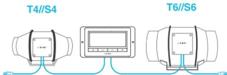
EC models can connect two fans of any size fan.
