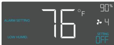
Note that alarm triggers can only activate in AUTO, ON, or TIMER Mode. Please leave ALARM SETTING to arm the controller.
