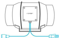
EC models have two cords with a molex connector and a three-pronged plug.
